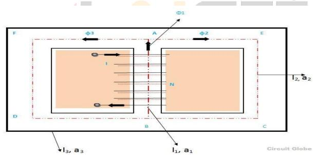
The above figure shows a parallel magnetic circuit.
